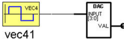
Figure 2. Application example of the Digital-Analog Converter
